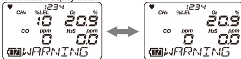
Display example Methane (CH4) concentration: 10 %LEL First alarm triggered
