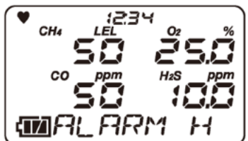
Third alarm setpoint display
